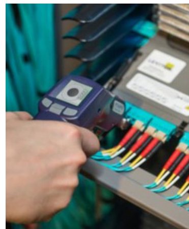
The FiberChek probe provides a fully automated handheld solution that makes inspection at the top of a cell tower fast and easy.
